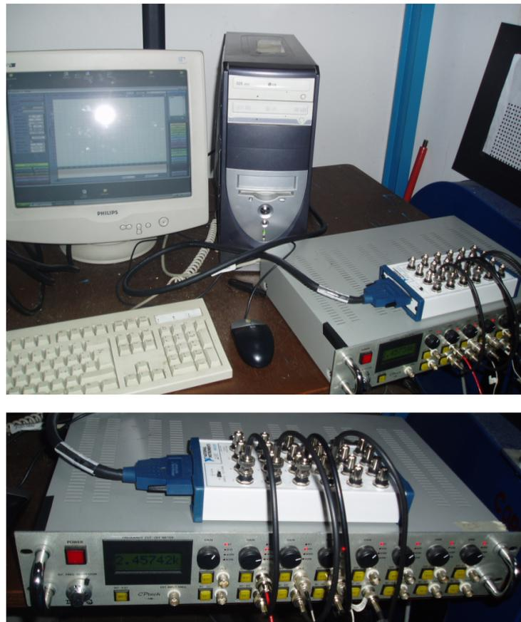
Figure 3-18: Data acquisition system involving the signal conditioner, data acquisition board and the PC.
