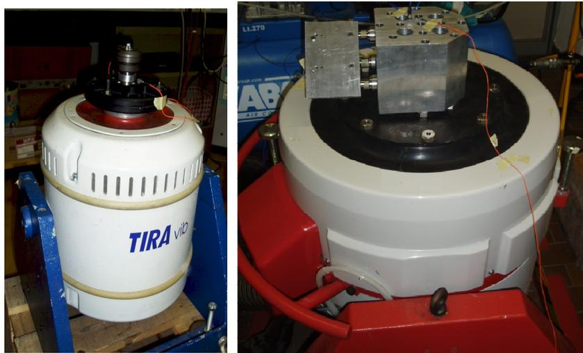
Figure 3-15: Vibration generators (shakers) used in the tests performed
