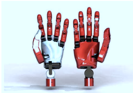
Figure 2.21: Rendered images of the 50% Female and 50% male 18 DOF Intrinsic hands and 3 DOF Intrinsic Wrists [91].
