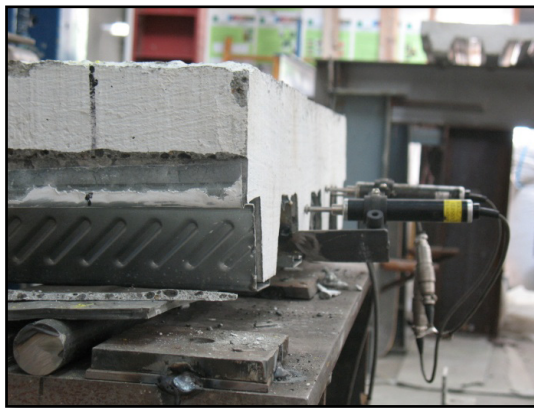
Figure 70 - Concrete end slip detail
