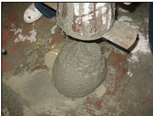
Figure 11 - Lift up the steel slump cone
