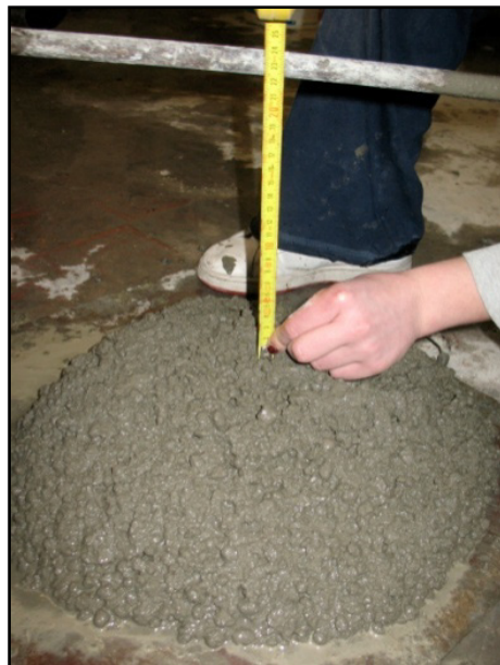
Figure 12 - Drop below the mould
