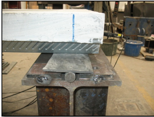
Figure 43 - Simple support carriage detail
