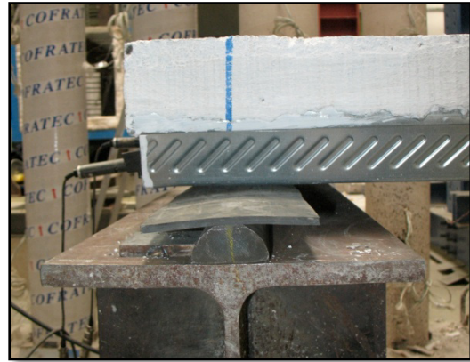
Figure 44 - Simple support hinge detail
