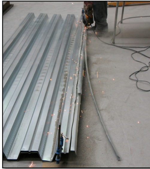
Figure 41 - Cut of profiled sheet
