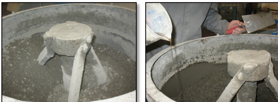
Figure 9 - Add of cement and superplasticizer
