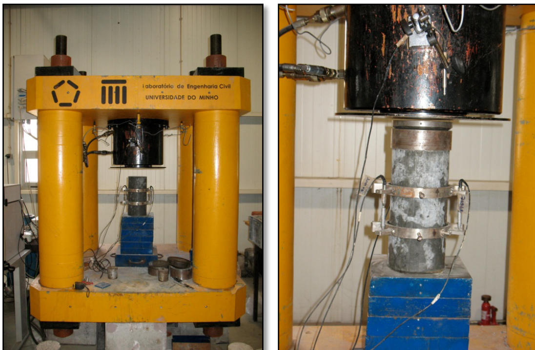
Figure 13- Modulus of elasticity testing machine
