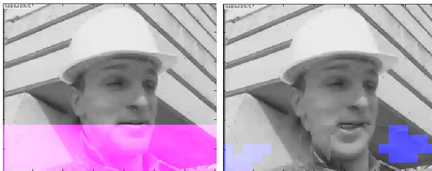
Figure 4.5: On the left the original noiseless frame with the lost slices in pink. On the right the corrupted and concealed frame with blue macroblocks perfectly restored. (Induced channel distortion equals to zero). The perfectly restored zones have uniform motion.
