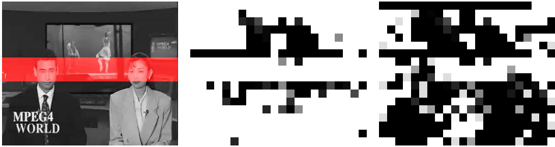
Figure 4.25: Starting from the left the corrupted video the likelihood map and the posterior map
