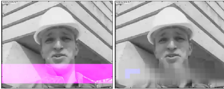
Figure 4.10: On the left the original noiseless frame with the lost slices in pink. On the right the corrupted and concealed frame with blue macroblocks nearly perfectly restored. The nearly perfectly restored zone is "Flat".
