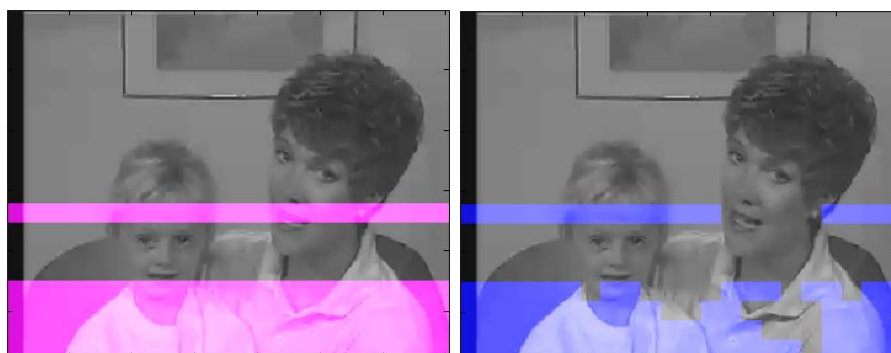
Figure 4.6: On the left the original noiseless frame with the lost slices in pink. On the right the corrupted and concealed frame with blue macroblocks perfectly restored. (Induced channel distortion equals to zero). The perfectly restored zones are "Flat".
