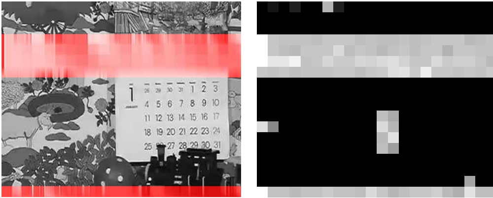
Figure 4.21: On the left the corrupted video, with lost slices in red, on the right the estimated likelihood map
