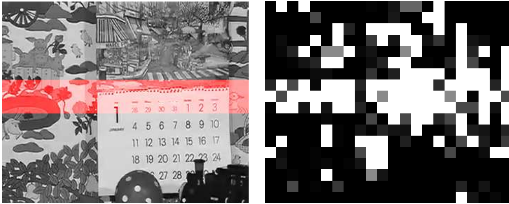
Figure 4.14: On the left the corrupted video, with the lost slices in red, on the right the estimated likelihood map
