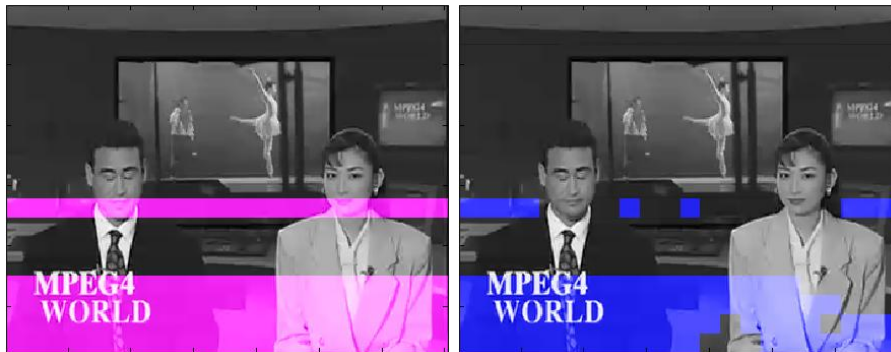
Figure 4.4: On the left the original noiseless frame with the lost slices in pink. On the right the corrupted and concealed frame with blue macroblocks perfectly restored. The perfectly restored zones have uniform zero motion. (Induced channel distortion equals to zero)
