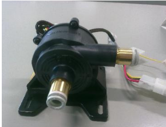
Figure 5-6: Example of a water circulating pump which is a part of the cooling system
