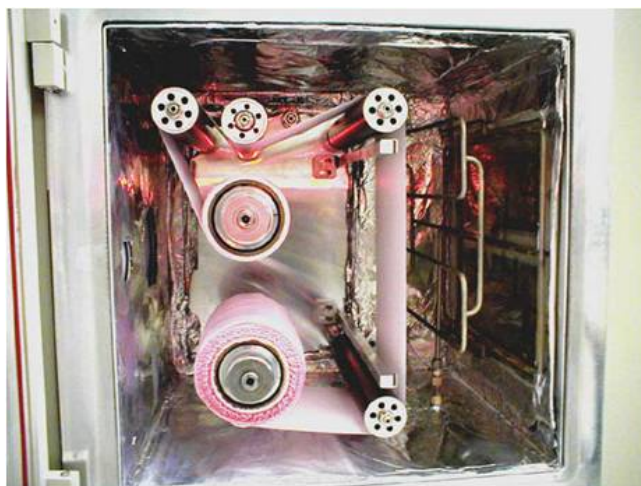
Figure 1.3: Basic idea of a roll-to-roll process: Unrolling the substrate, processing, rolling again. The high throughput and low cost of such systems are perfectly tuned with PV industry requirements.
