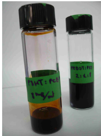
Figure 2.3: PEDOT:PSS (blue) and P3HT:PCBM (red) solutions.
