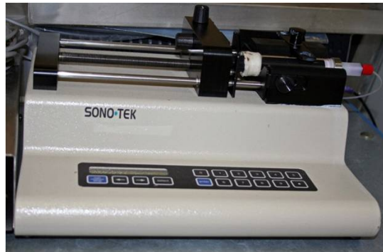
Figure 2.8: Solution loaded in a syringe, ready to be sent to the nozzle through a small pipe by mean of an electromechanical dispenser.
