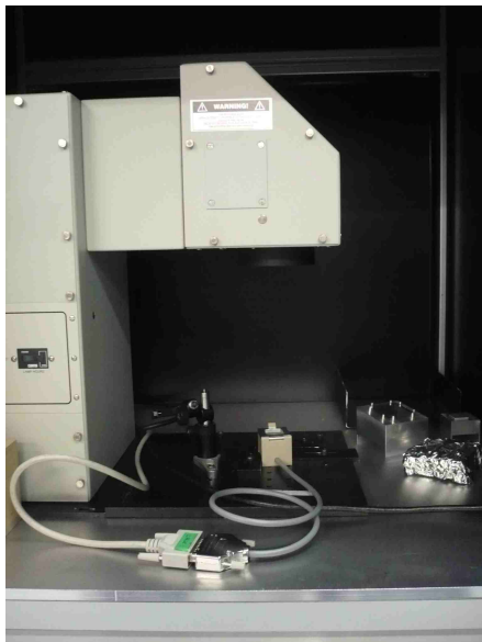
Figure 2.6: Solar simulator for organic solar cells testing. The illumination of the lamp refers to 1 sun AM 1.5 spectrum.
