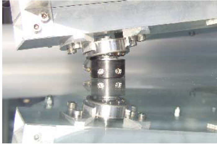
Figure 2.5: Nelson air airbearing binded to SKF ball bearing
