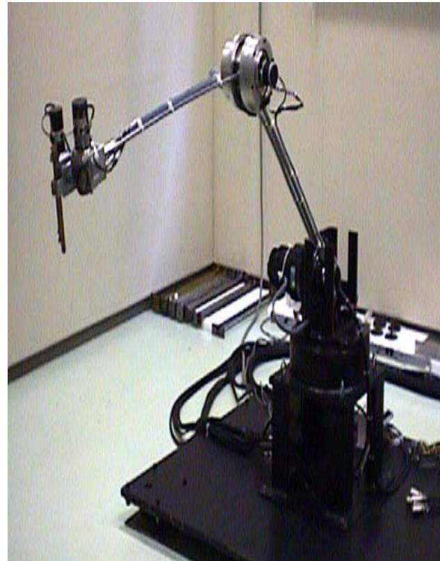
Figure 1.4 A manipulator with flexible links
