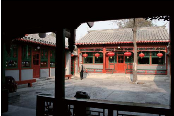
Figure 50: Courtyard is larger in the cold climate zone (north of China) to gain more sunlight in winter
