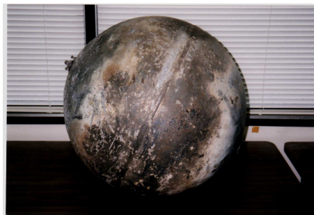
Figure 2.34: A 30 kg titanium pressurant tank from Delta 2 second stage reentered the atmosphere in Texas, US
