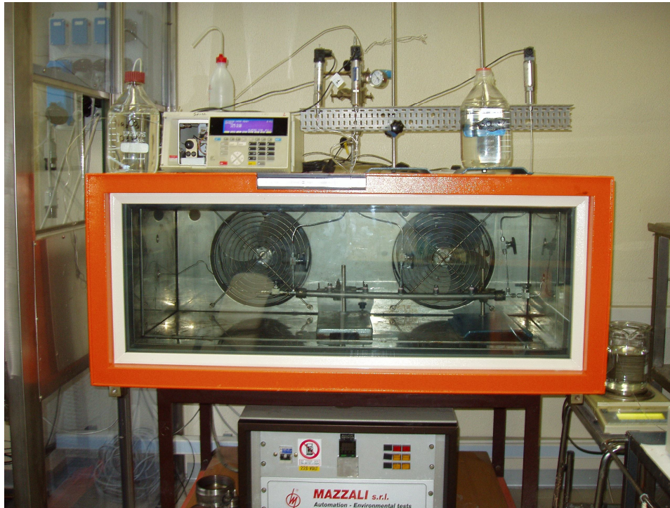
Figure 7-3 – Instrumentation used for core flooding
