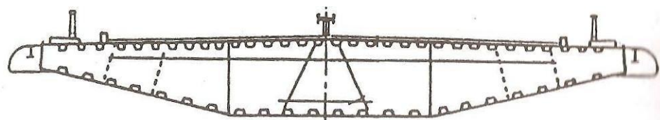
Figure 5: The Normandy Bridge cross-section: an aerodynamic profile. Figure from [7]
