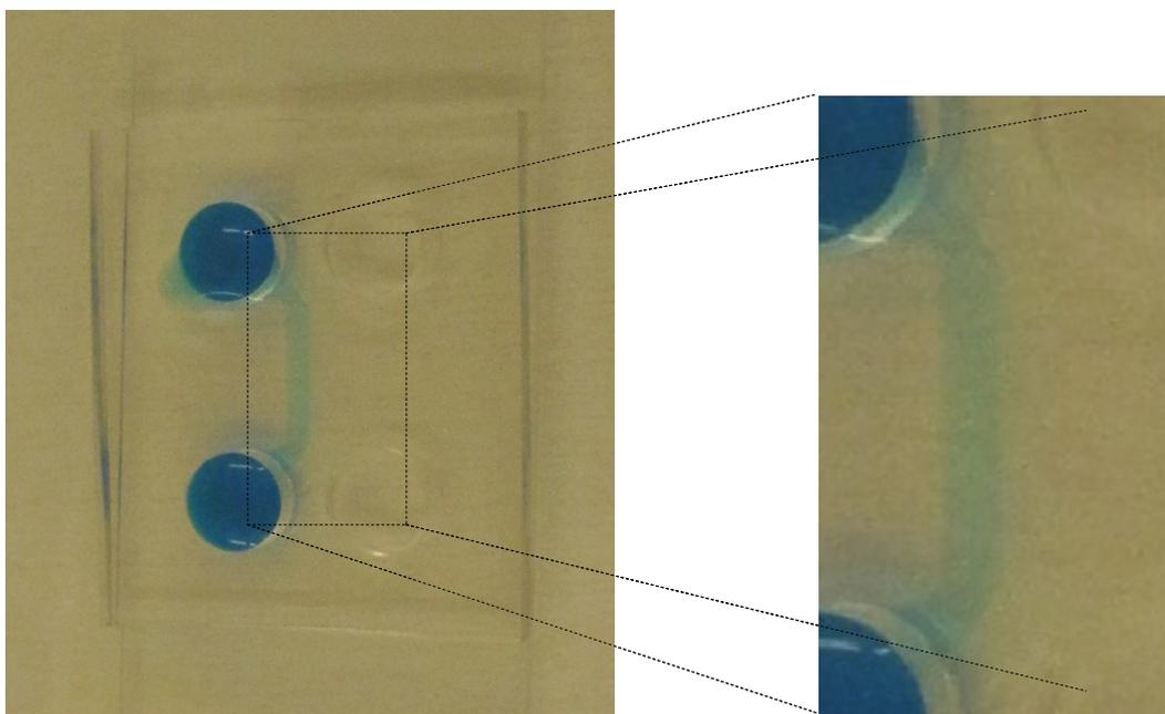
Figure 27: PDMS full with blue food additive in one compartment and water in the other
