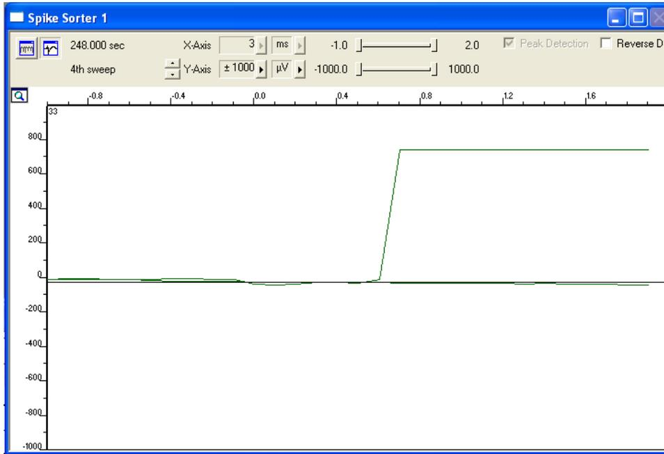
Figure 43: Saturation effect on electrode 33 during stimulation in electrode 85 without external ground; [values: x-axis in ms, y-values in  $\mu\text{V}$ ]
