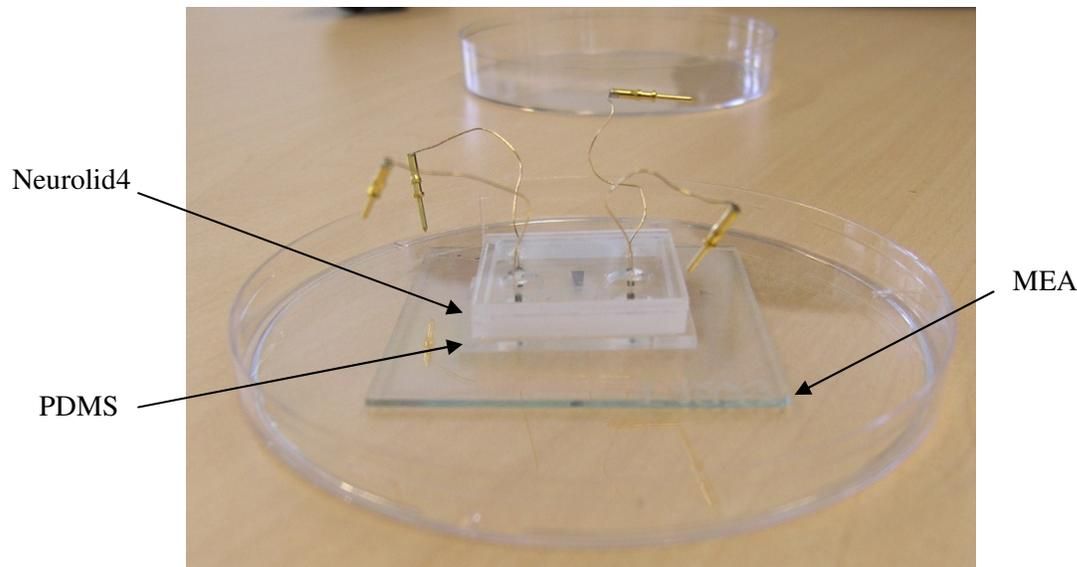
Figure 13: The complete scheme highlighting the three layers
