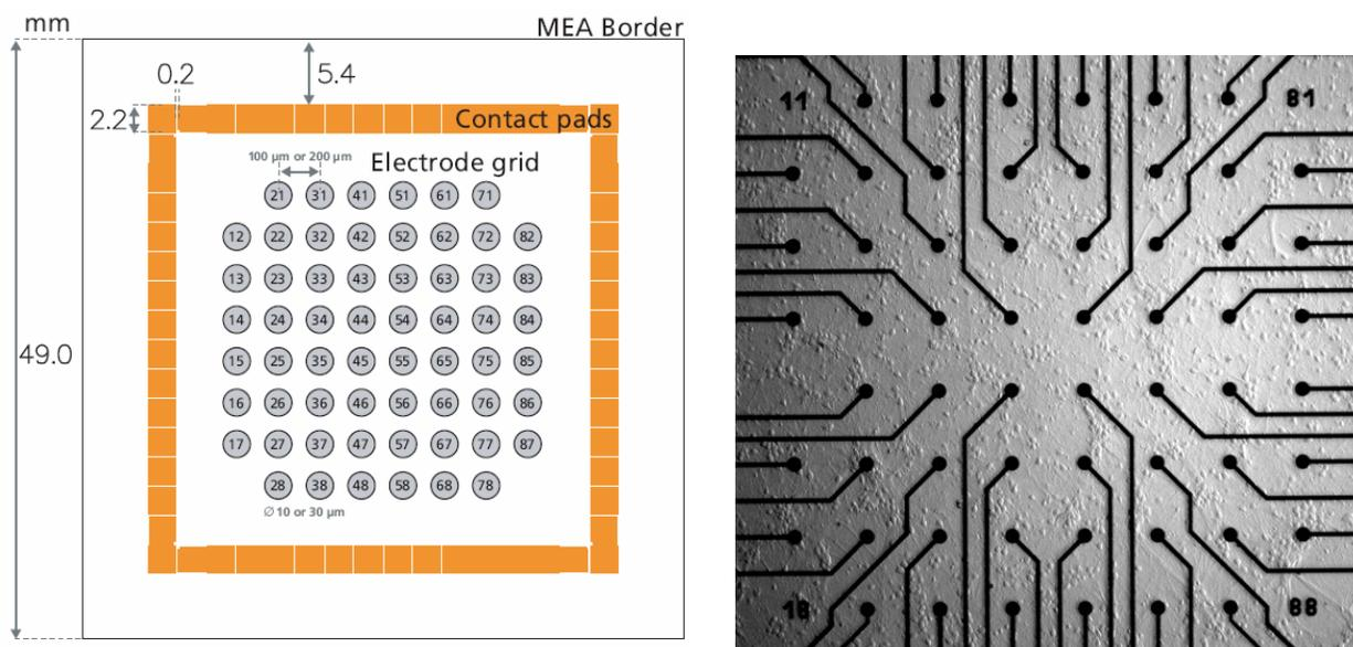
Figure 1: A\_ Model of the MEA array with electrodes number in the 8x8 grid; B\_ A real photo of one device.
