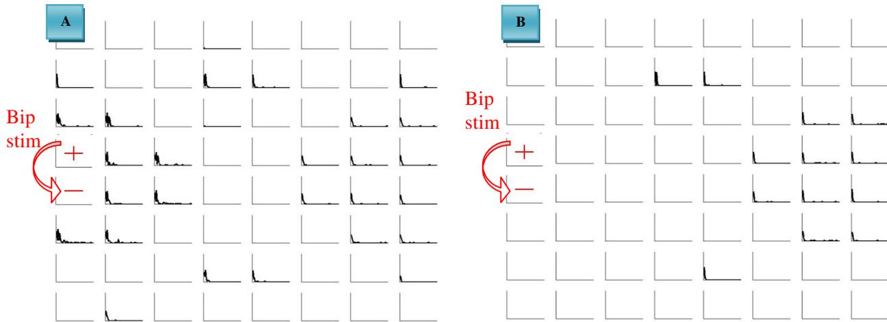
Figure 57: PSTH analysis of Bipolar electrical stimulation in compartment A (Device #: 46\_I1377\_24); Stimulation was applied across electrode 14 (e14) and 15 (e15) with 4 external electrodes; A: Stimulation without TTX in any compartment; B: stimulation with TTX in compartment A
