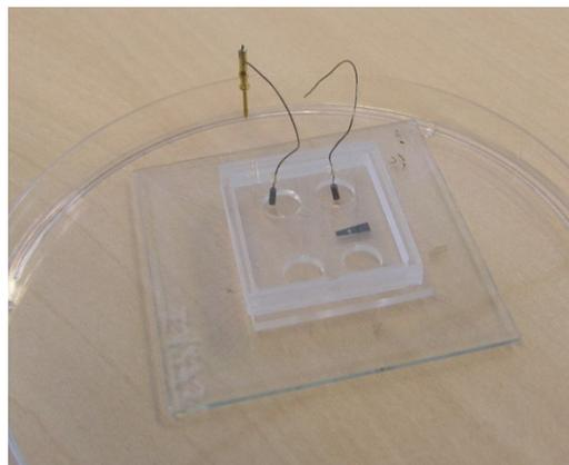
Figure 10: Neurolid2 put on the PDMS – 1 grounded electrode per each compartment
