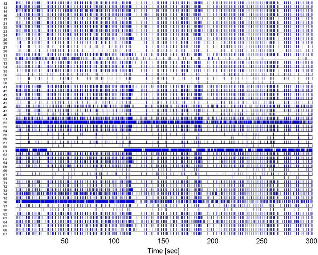
Figure 20: Raster Plot of an active device; y-axis represents the number of the electrode (Device #: 41\_12549\_24: Spontaneous activity)
