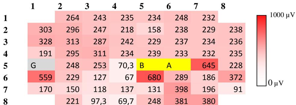
Trials were then done changing the positions of the two external grounded electrodes.
