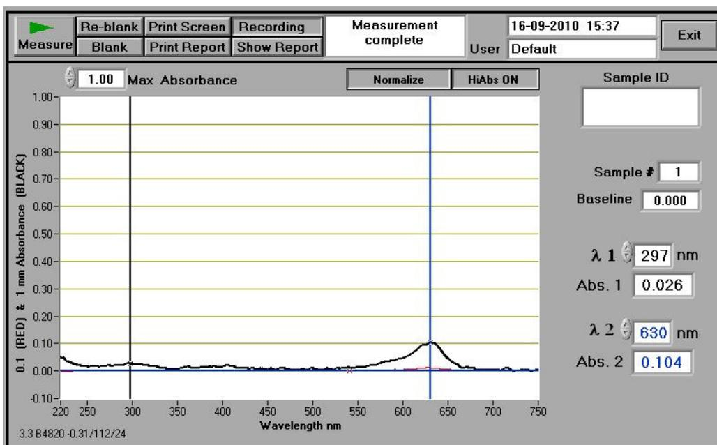
Figure 29: Spectrophotometer of H<sub>2</sub>O after 24 hours in compartment A in a PDMS where the compartment B contained a blue food additive.
