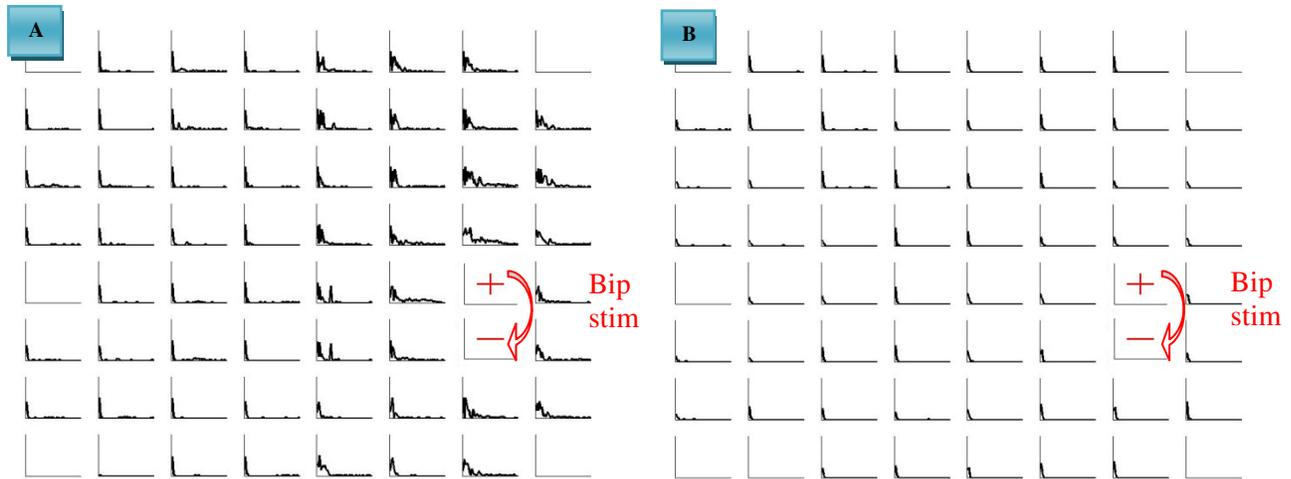
Figure 55: PSTH analysis of bipolar electrical stimulation on a device on DIV 22 (Device #: 46\_14589\_22). Bipolar stimulation was applied across the electrodes 75 (e75) and 76 (e76) with 4 External Grounded Electrodes; A: PSTH analysis of bipolar stimulation without TTX in any compartment; B: PSTH analysis of bipolar stimulation with TTX in compartment B
