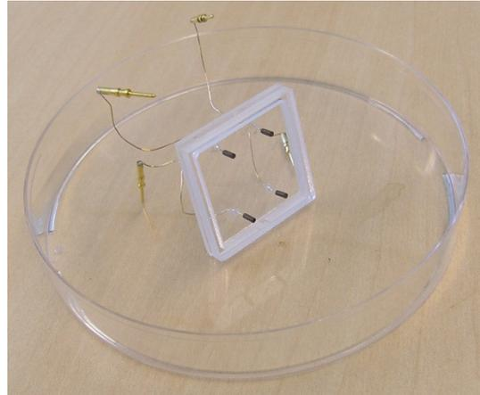
Figure 11: Neurolid4: neurolid with 4 electrodes
