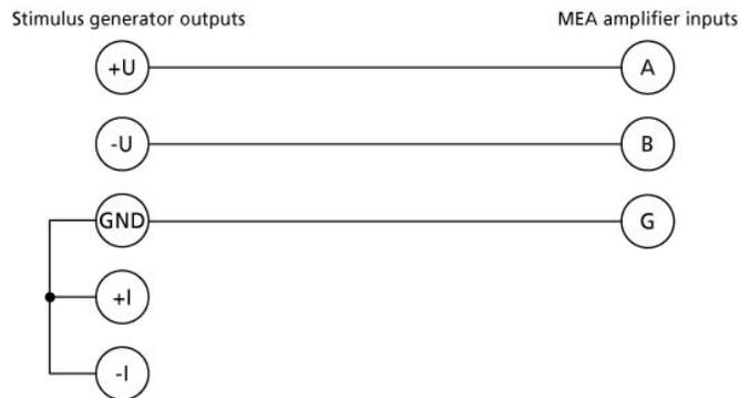
Figure 16: Standard setup for bipolar stimulation
