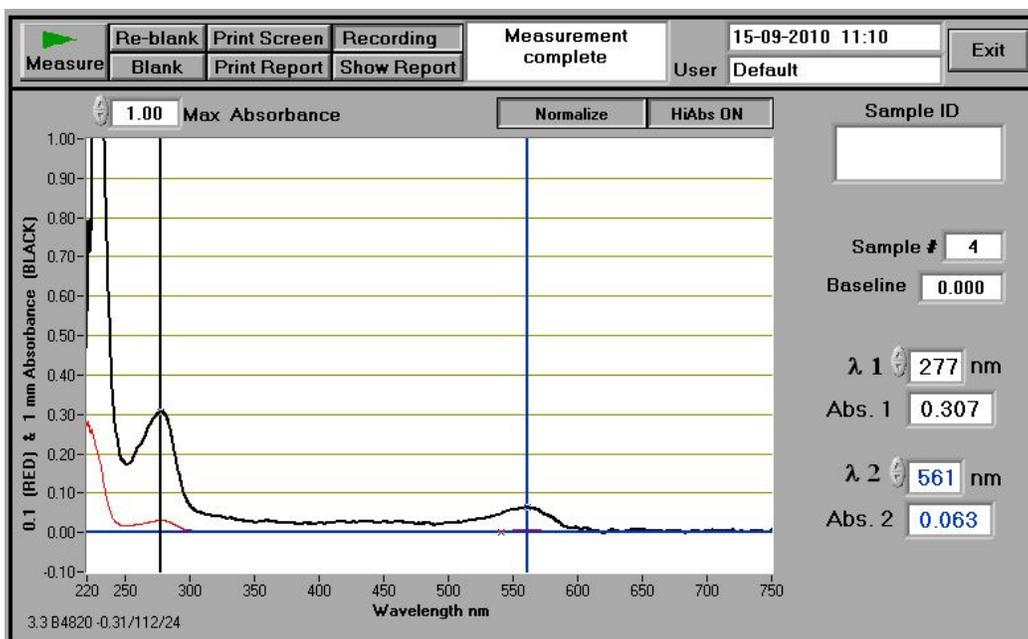
Figure 25: Spectrophotometer of neural medium with a concentration of 100nM of TTX
