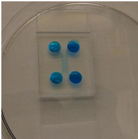
Figure 3: Photo of a PDMS filled with a blue food coloring substance to highlight the shape of the micro-channels
