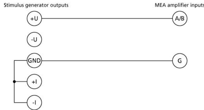
Figure 15: Standard setup for unipolar stimulation
