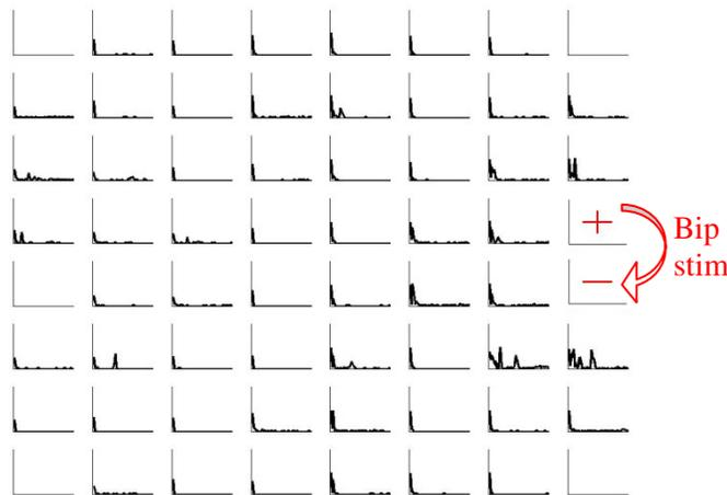
Figure 56: PSTH analysis of Bipolar electrical stimulation in compartment B (Device #: 46\_11377\_24); Stimulation was applied across electrode 84 (e84) and electrode 85 (e85) with 4 external electrodes.
