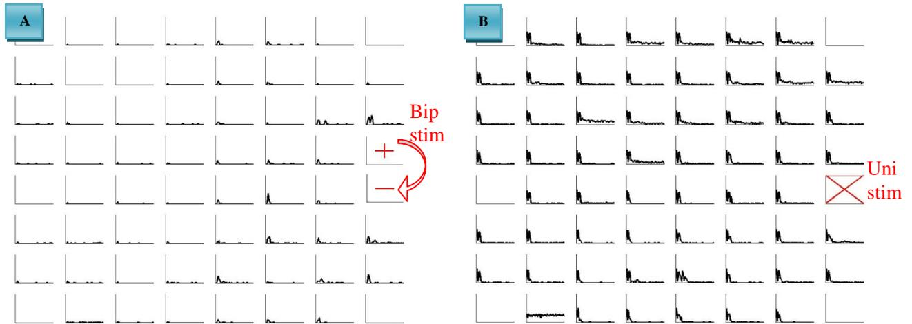
Figure 59: PSTH analysis to show confirm focused bipolar electrical stimulation (Device #: 46\_12550\_DIV25) with 4 external reference electrodes and after removing artifacts from the recordings; A: Bipolar stimulation of electrode 84 (e84) and electrode 85 (e85) in compartment B; B: Unipolar stimulation of electrode (e85) in compartment B
