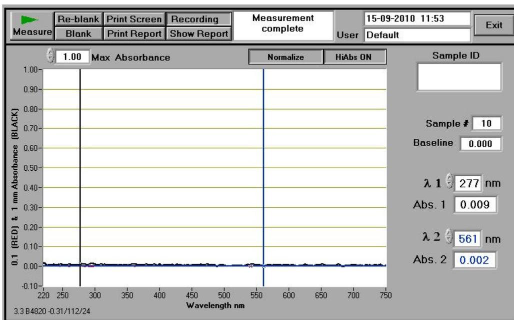
Figure 28: Spectrophotometer of H<sub>2</sub>O after 15 minutes in compartment A in a PDMS where the compartment B contained a blue food additive, easily detectable by the spectrophotometer
