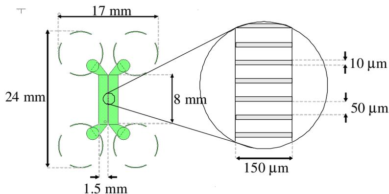
Figure 2: Schematic layout of dual compartment device design used for neuronal cell culture; A- Reservoir (diameter=6mm), B and C – Dual compartments (width=1.5mm, height=0.1mm, length=8mm), D – Micro-channels (width=10µm, height=3 µm)
