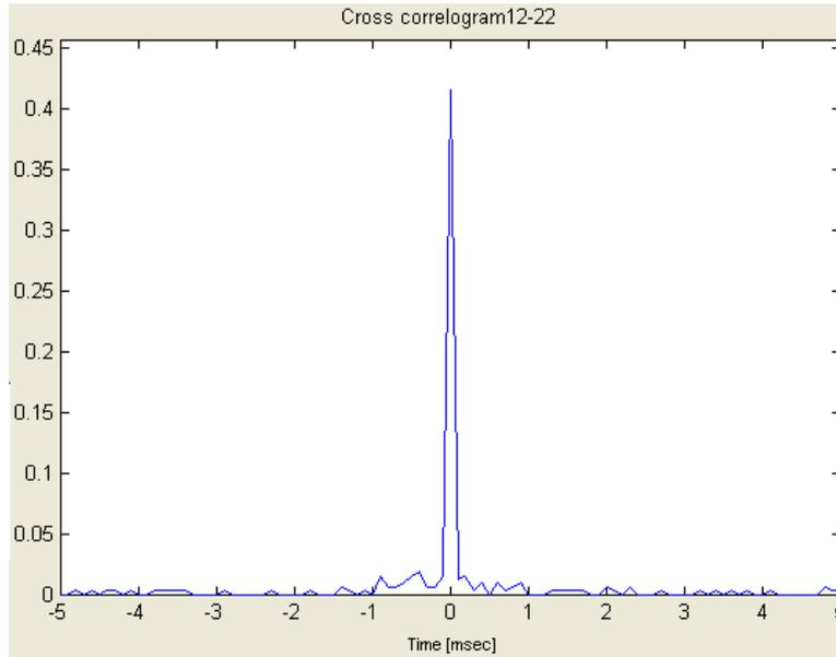
Figure 6: example of correlation between electrodes 12-22; [values: x-axis -5:+5 ms; y-axis probability of correlation]
