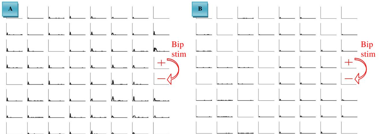
Figure 58: Influence of TTX on network activity. PSTH analysis of Bipolar electrical stimulation of electrode 84 (e84) and 85 (e85) in compartment B on DIV 22 (Device #: 46\_12550\_DIV22) with 4 external reference electrodes and after removing the artifacts from the recordings; Figure 6A: Without TTX in any of the compartment; Figure 6B with TTX in compartment B
