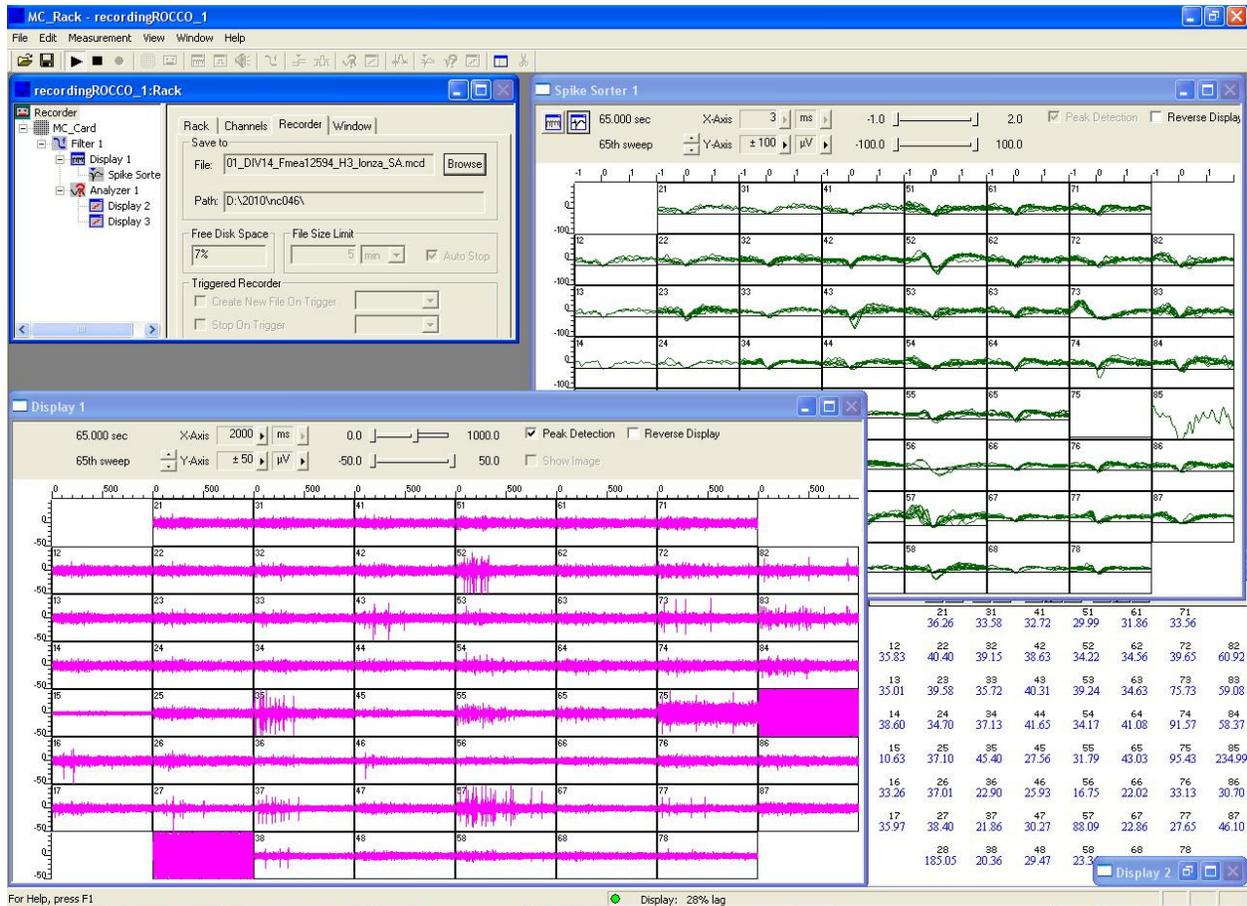
Figure 17: MCRack screenshot of an active culture; electrodes 28 and 85 are considered to be noisy
