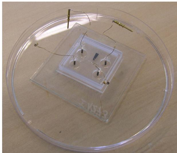
Figure 12: Neurolid4 put on the PDMS – 2 grounded electrode per each compartment (1 per reservoir)
