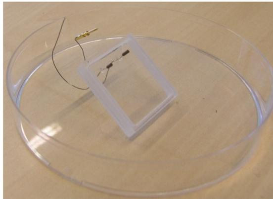
Figure 9: Neurolid2: neurolid with 2 electrodes
