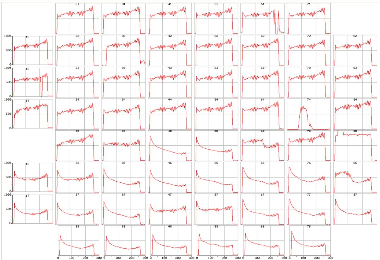
Figure 42: Artifacts history during stimulation of electrode 85 and ground in electrode 15 and neurolid2; electrode 74 is noisy [Values: x-axis 0-300 seconds, y-axis 1000  $\mu\text{V}$ ]
