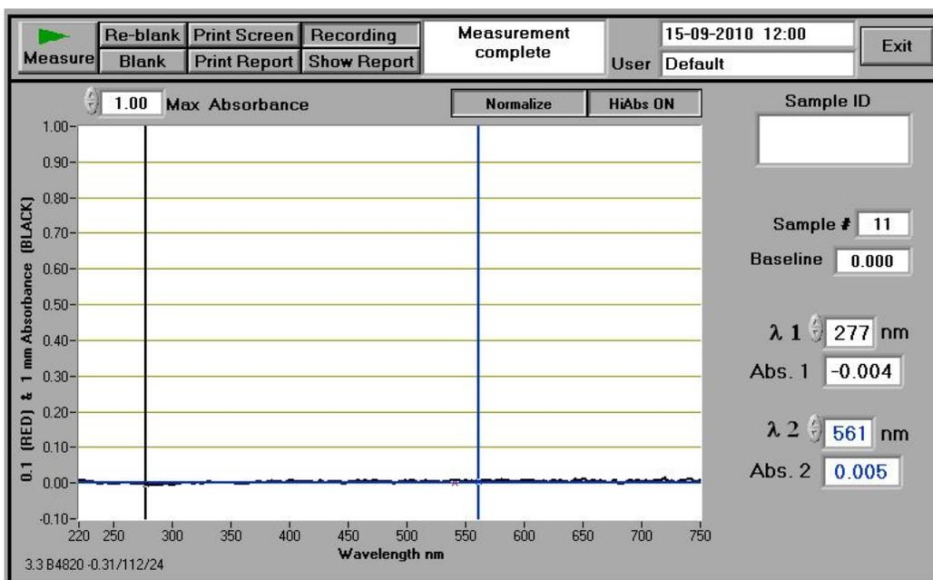
Figure 31: Spectrophotometer of H<sub>2</sub>O after 15 minutes in compartment A in a PDMS where the compartment B contained a neural medium. The neural medium was left before 15 minutes in compartment B with an empty compartment A
