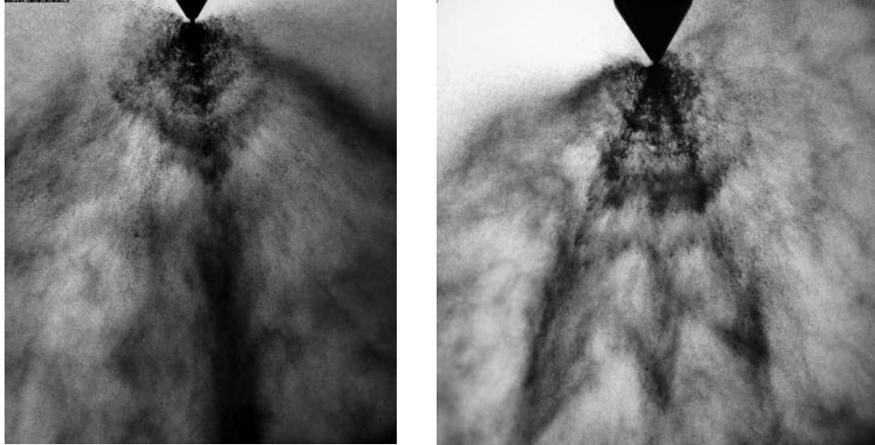
(a) Decane ( Oh=0.0076 ) U_j = 79.3m/s , Re = 39576 , We = 134071 (b) 1-Hexene ( Oh=0.0027 ) U_{jet} = 67.6m/s , Re = 110141 , We = 112527
