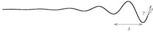
Figure 2.4: Liquid sheet sketch y(r, t) close to the rim showing a primary undulation of wavelength \lambda and the component \gamma of the acceleration
