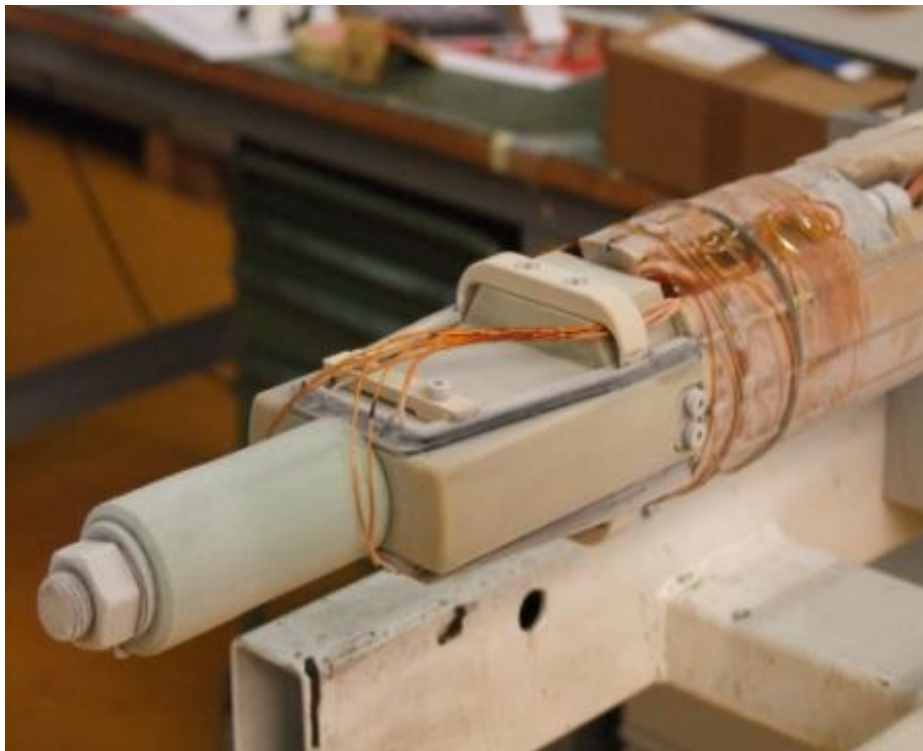
Figure 57. The (frozen) shaft after its extraction from the cryostat during the first tests of the SIT sample holder. The black strip along the U is the layer of polymeric glue that has been put to totally fix the wire. This figure also shows the two sets of voltage taps (copper filaments) connected to the basis of the sample holders.
