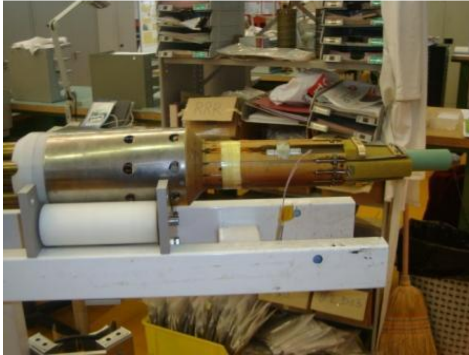
Figure 56. Installation of the two SIT sample holder prototypes on the CERN measurement shafts, thanks to the new mechanical support, that has been designed to test both prototypes using a single shaft.
