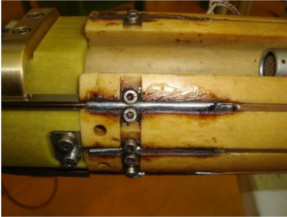
Figure 58. The soldering strip on the electric connection between the current leads during the sample holder preparation.
