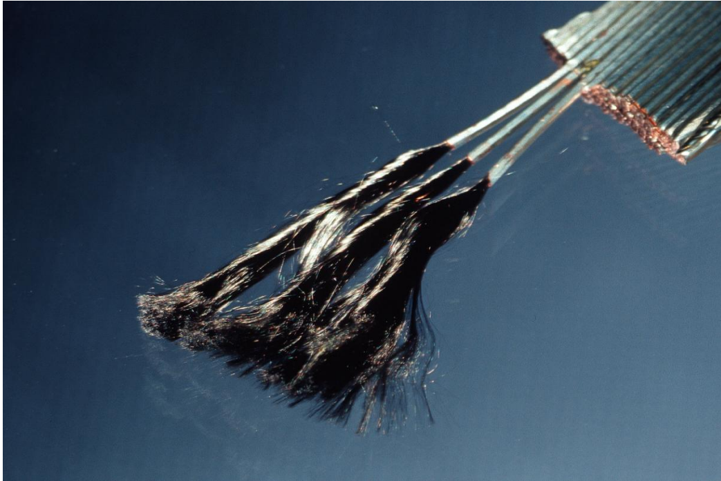
Figure 15. Internal structure of a Rutherford Cable, that has been built with NbTi wires. NbTi filaments come out of the three wires, that have been “isolated” on the cable. Acknowledgements: Christian Scheuerlein (CERN - TE - MSC group).
