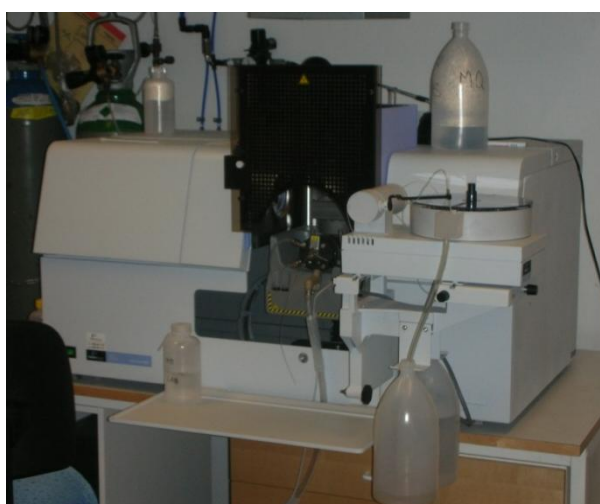
Fig.4.15: The atomic absorption spectrometer, a Perkin Elmer AAnalyst 800, used to analyse released metal concentrations at the Division of Surface and Corrosion Science, KTH.
