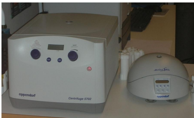
Fig.4.14: Picture of the two centrifuges (Eppendorf Centrifuge 5702 and Eppendorf Minispin) used to separate any particles from the test media after the electrochemical measurements performed within this work.
