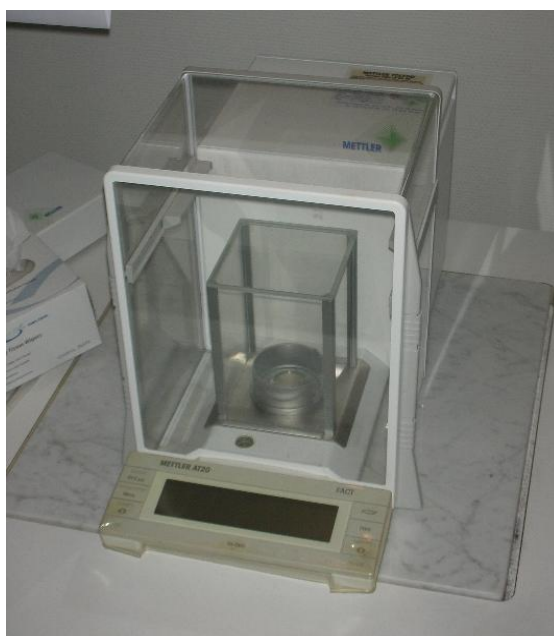
Fig.4.8: The Mettler AT20 microbalance used to weigh the 316L stainless steel particles.
