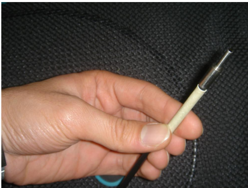
Fig. 3.16. Asd Inc © Fieldspec plug to capture information about one precise region
