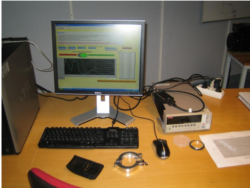
Fig. 5.7 Data acquisition desk. The source-meter is placed on the right of the computer screen.
