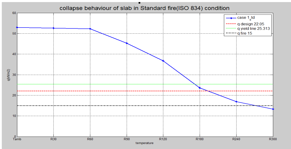
Figure 26: Actual collapse load of the slab in standard fire condition, only case 1.
