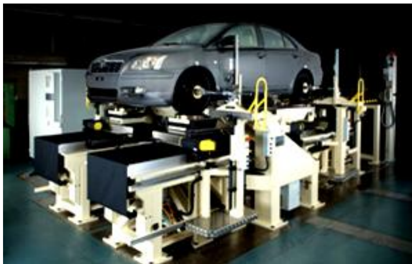
Figure 6 - Suspension Parameter Measurement Machine (SPMM).
