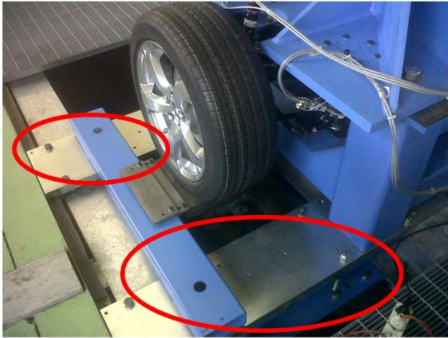
Figure 10 – Beams Limiting the Available Space for Rolling Road
