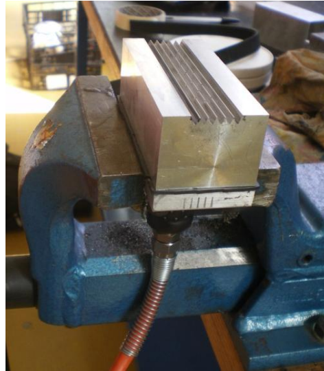
Figure 37 - Air Bearing Experimental Test Setup
