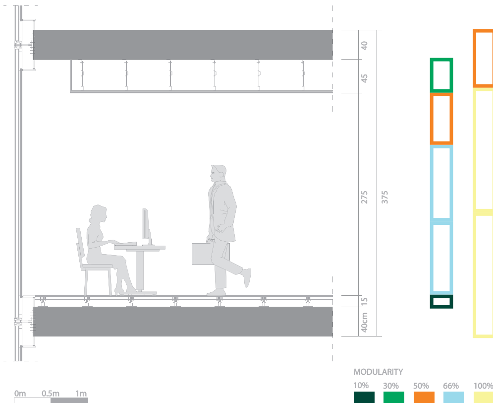
Drawing 21: Section illustrating the use of modularity to design the height of used spaces and total height of each floor. Scale indicated.
