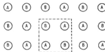
Fig.5.9 Unit cell base in disordered structure of a binary alloy; two types of atoms in the base
