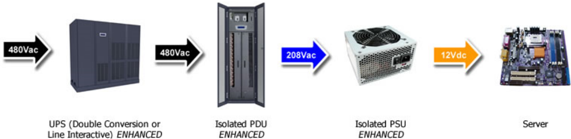
Figure 7 480V-208V Power Distribution scheme
