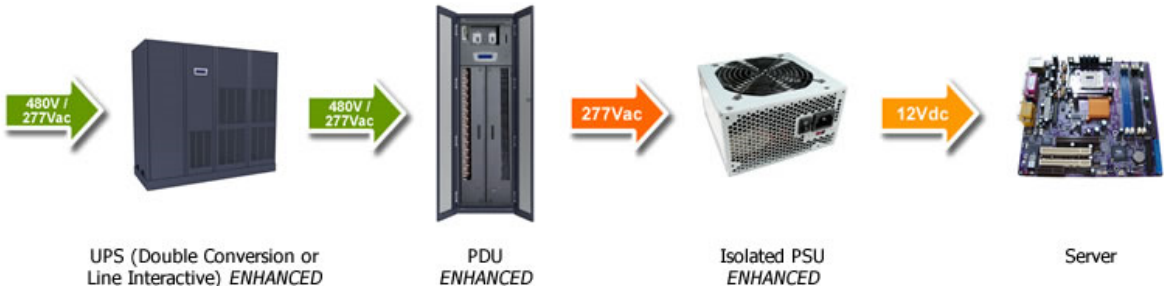
Figure 8 480V/277V Power Distribution scheme
