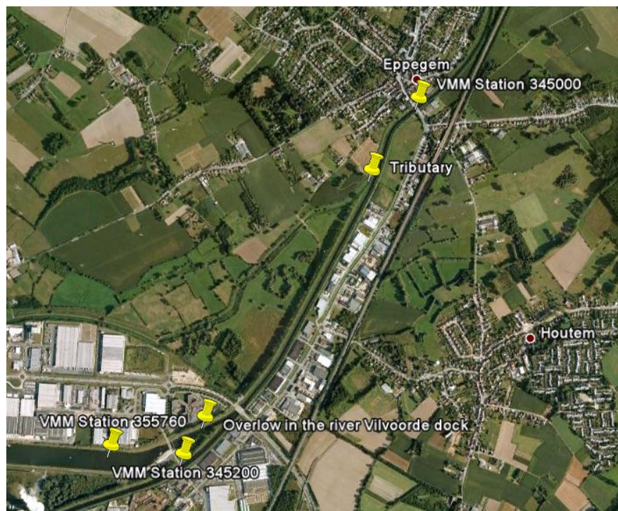
Figure 65 Overview of the overflow in Vilvoorde dock and the measurement station of the VMM used to analyze the difference in water quality upstream and downstream the overflow
