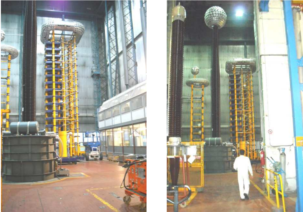
Figure 7: Test room SPE (in background device simulating wet test)
