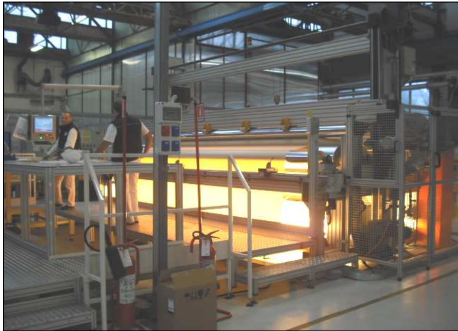
Figure 5: Winding machine in phase of paper drying
