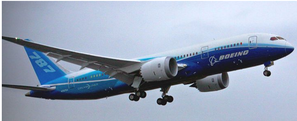
Figure 1.1: Boeing 787: the world's first major airliner to use composite materials for most of its construction.
