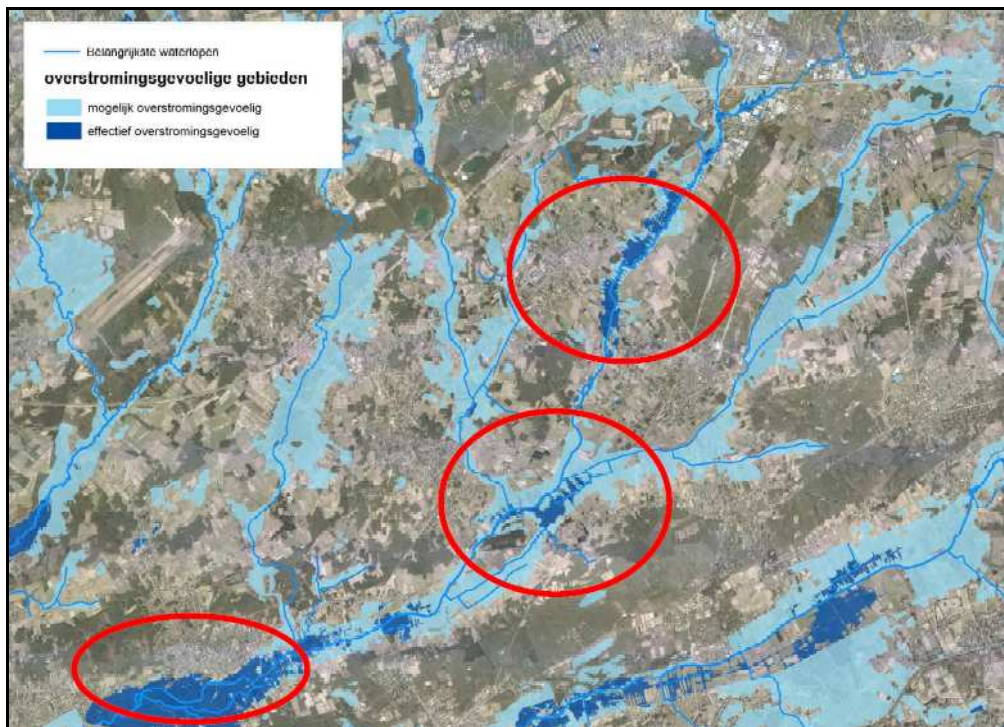
Figure A.9: the potential (light blue) and effective (dark blue) flood prone areas (red circle) along the lower Aa valley (adapted from Abrams, 2009).
