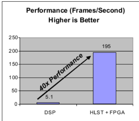
Figure 2.13: Maximum frame rate achieved for a video application on a DSP processor and an FPGA plus HLS tools.
