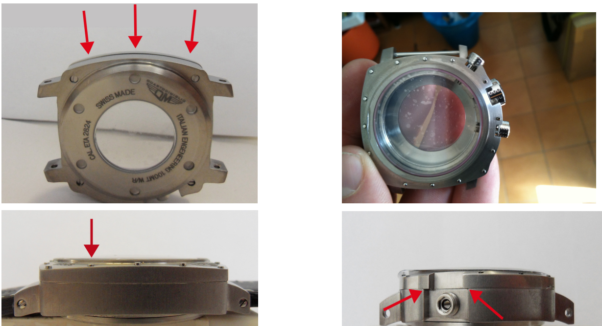
Illustration 4.4.2: Example of defects on the case and on the glass of the watch
