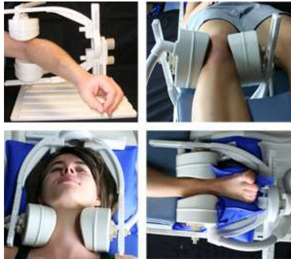
Figure 1.6: Example of a surface coils that offers a wider selection of positioning options and It enables the examination of joints in stretched or bent positions ( Noras MRI products, http://www.noras.de )
