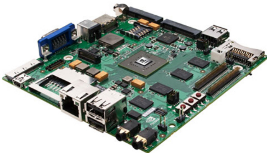
Figure 5.2: NVIDIA Tegra 250 developer kit. The SoC is only the square in the centre, while the other ports are expressly designed for the development board.
