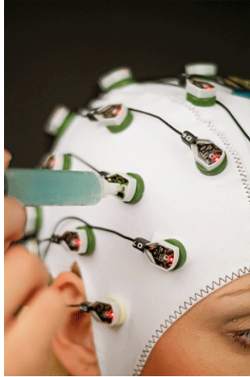
Figure 3.8: Electrodes placement in EEG examination. It is obvious that this kind of sampling procedure is unsuitable for HCI
