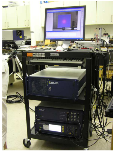
Figure 4.6: Vibrometer controller and data management system
