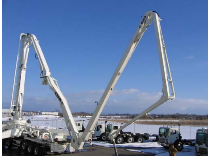
Figure II.1: Example of mobile application of booms for concrete handling.
