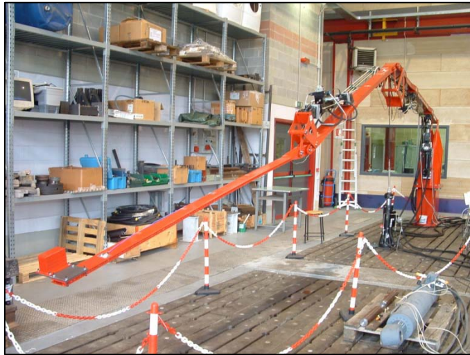
Figure 2: Example of mobile application of booms for concrete-handling
