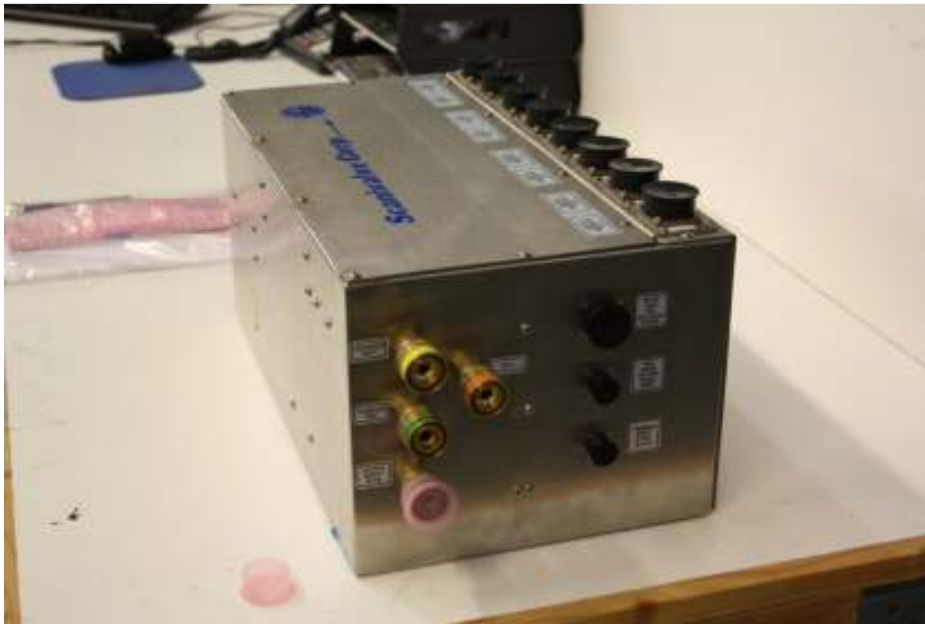
Figure 48 - Scanivalve which contains the pressure transducer device
