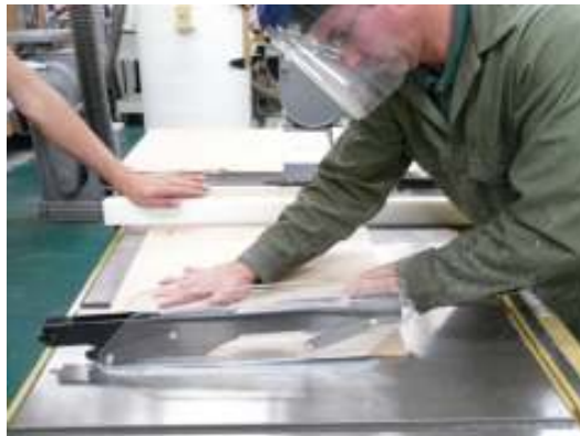
Figure 37 - Cutting the plexiglass
