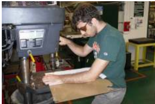
Figure 36 - Drilling the holes
