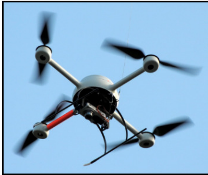
Figure 1.2 – Microdrones MD4-200 with amateur camera as image sensor
