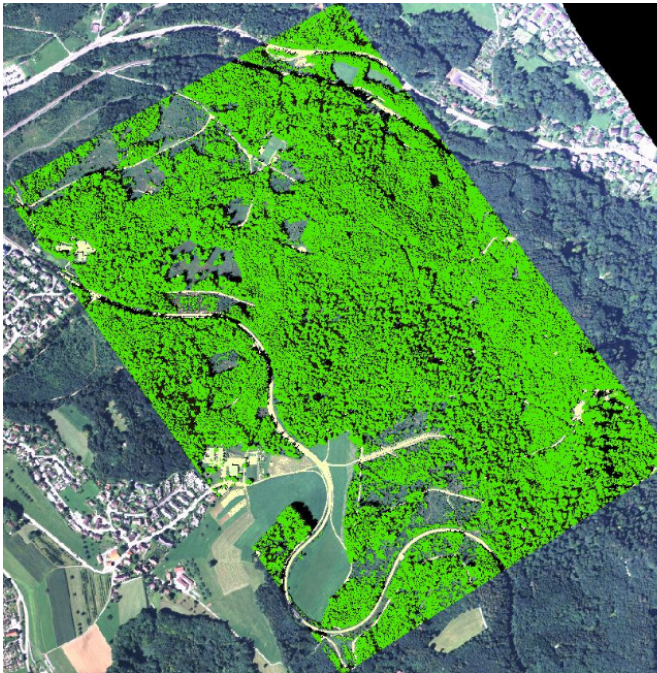
Figure 5.7 – Tree mask overlaid on the RGB orthophoto
