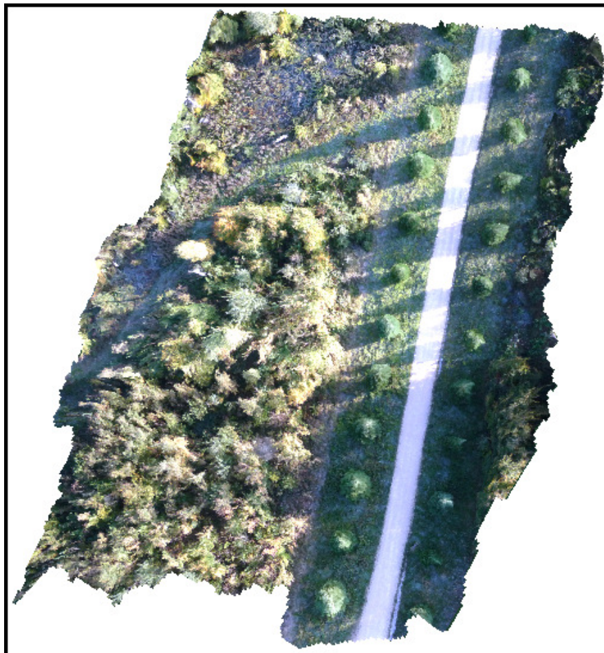
Figure 3.28 – Mosaicing of the orthophotos generated by the DSM: outliers and blur's effects are especially present at the edges
