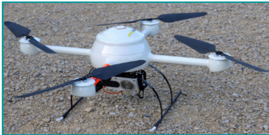
Figure 2.5 – The Panasonic Lumix DMC–FX35 camera, mounted on the Microdrones MD4-200
