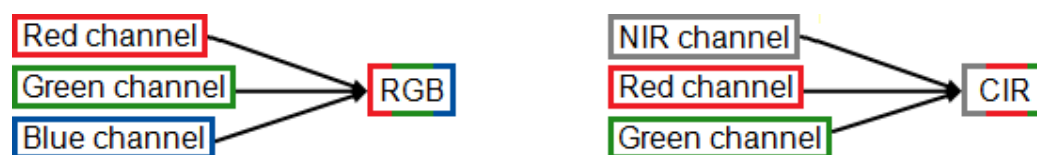
Figure 5.3 – Channels combinations: Red Green Blue (RGB) and Color Infrared (CIR)
