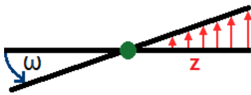
Figure 3.18 – Variation of the Z coordinate, which increases with the distance from the central GCP (in green)
