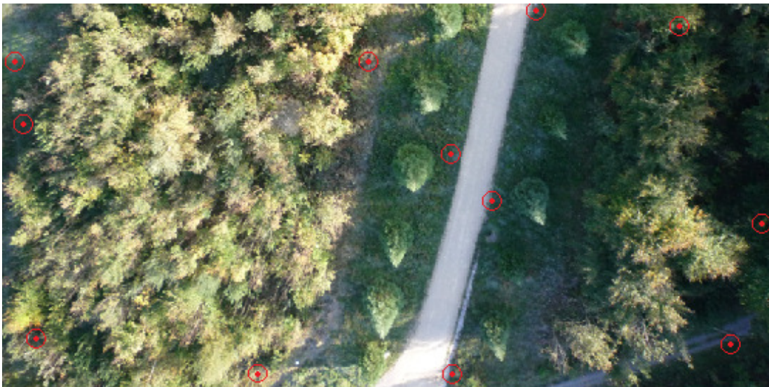
Figure 3.9 – Distribution of TPs (red dots in the circles) in the overlap area between images 615 and 618
