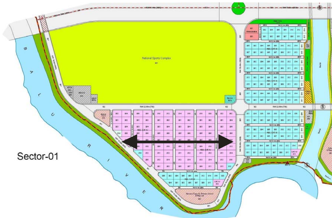
Figure 6.4: Building Orientation along the River (East-West Direction) In proposed layout plan of new city Purbachal, (At Eastern Fringe, Dhaka)
