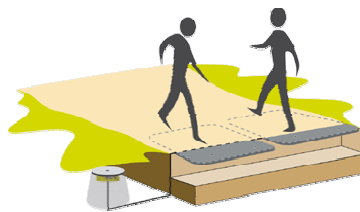
Figure 2- 10: Pressure-sensitive Mats Feel the Weight
