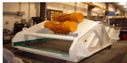
Fig: Dewatering Screen
