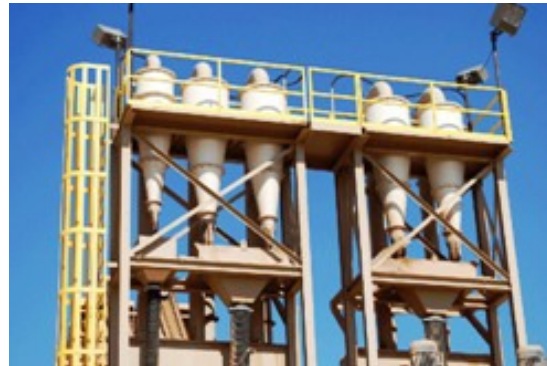
Fig: Super cutter Hydrocyclone
