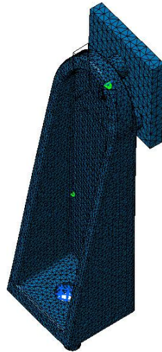
Figure 3.18 Lens 3 support under FEM investigation.
