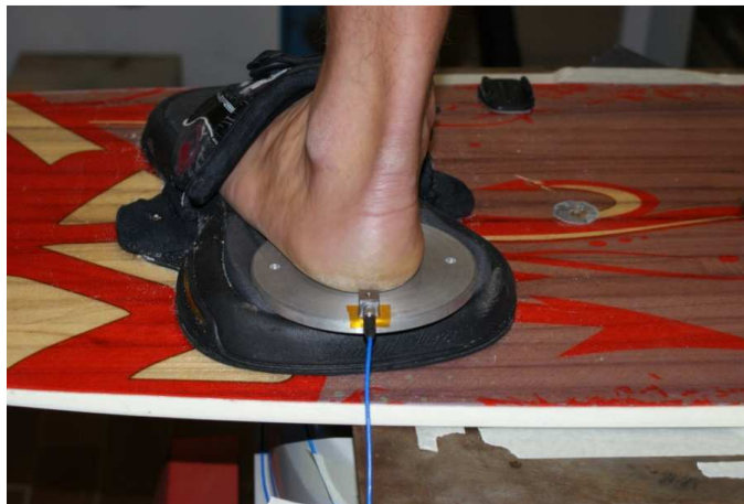
Figure 4.3 Position of the third accelerometer to measure the vibration on the heel, vibration entering the body.
