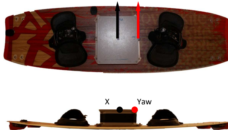
Figure 5.4 Position of the triaxial and monoaxial accelerometers for the measure of the yaw, triaxial (black) monoaxial (red).
