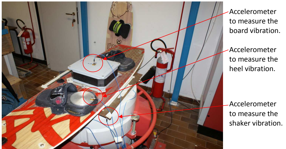
Figure 4.1 Position of the accelerometers during the test with the aluminium box.
