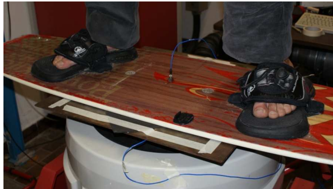
Figure 4.2 Position of the second accelerometer during the test without the aluminium box.
