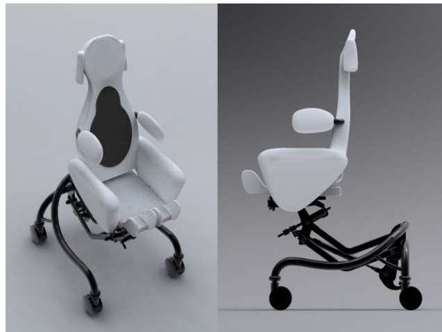
Picture 23 Virtual representation of the seating system (without coating).
