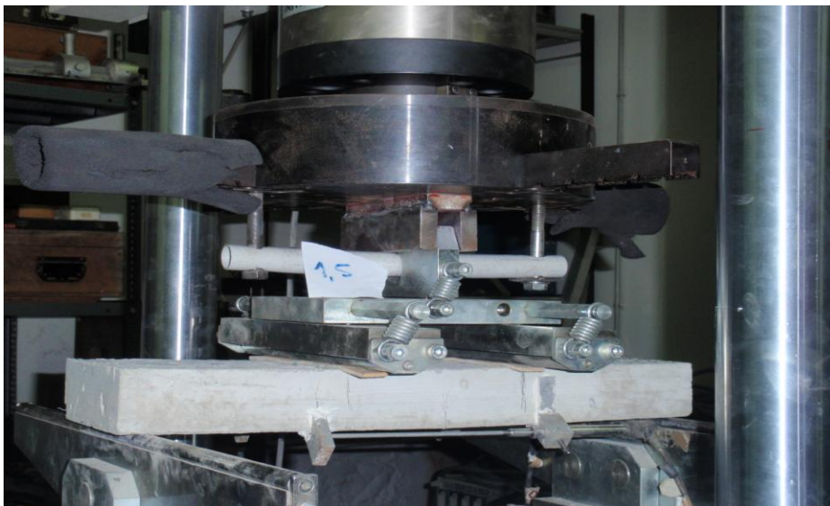
Figure 4.16 bending test set up,
