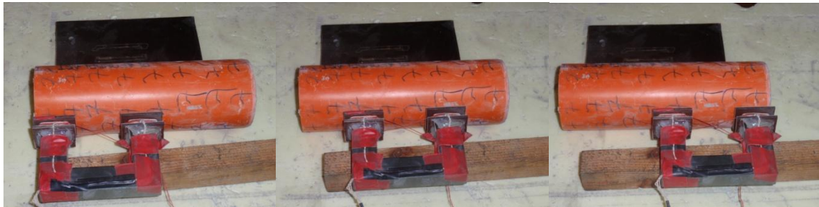
Figure 4.13: cylindrical samples with magnetic probe.
