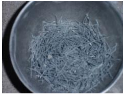
Figure 4.15: the steel fiber as crashed out of hardened concrete and collected in a can.
