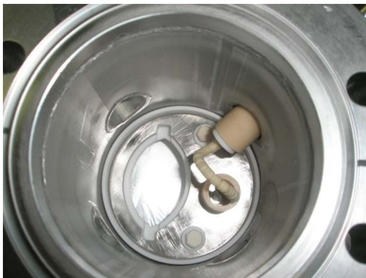
Figure 79: insight of the sample holder and power feedthrough.
