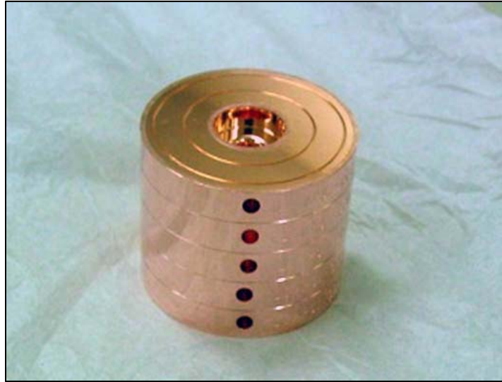
Figure 40: Five-cells bonded structure.
