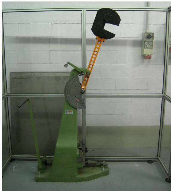
Figure 3.9: Charpy pendulum for Impact tests presents at Falco laboratories (Politecnico di Milano).
