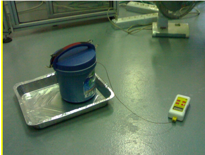
Figure 3.7: Image of the insulated vessel for Charpy specimens cooling whose temperature is controlled by a thermocouple.
