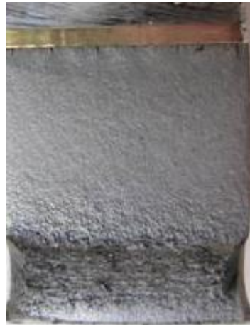
Figure 5.4: Optical image of the fracture surface of X65 steel H-free, investigated in Figure 5.5.
