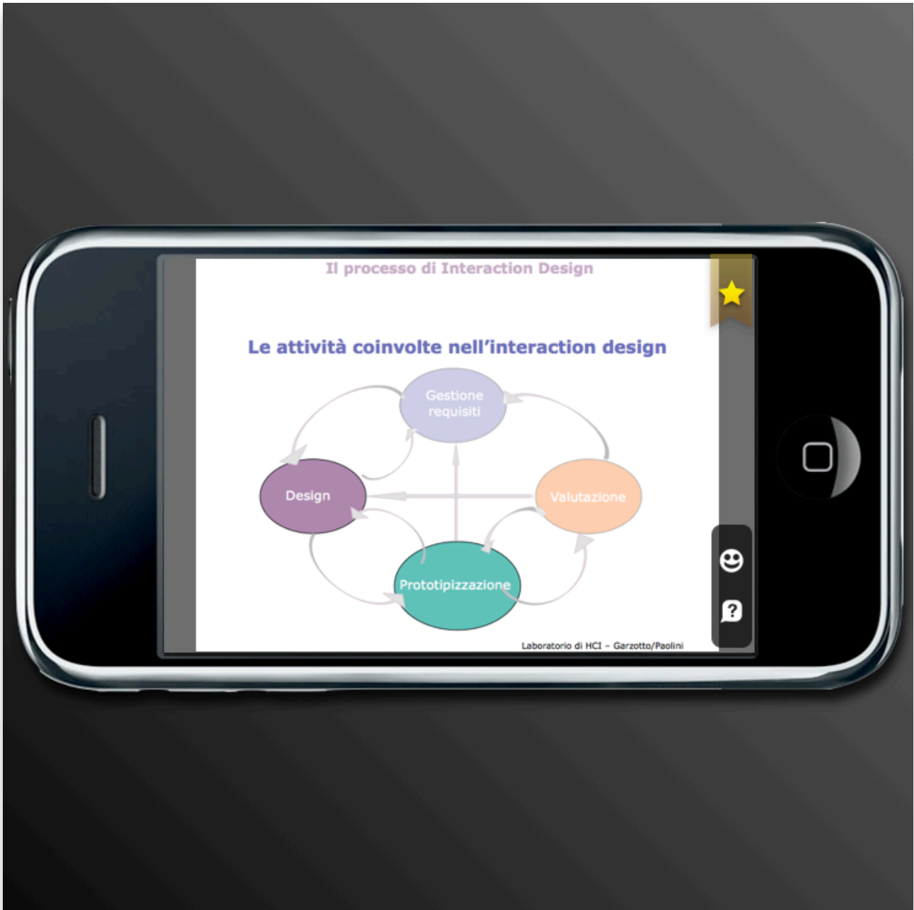
Figure 7.4: In landscape mode, controls are made vertical to avoid content interference. A “ribbon” control allows for quick highlighting of the entire slide as “important”.
