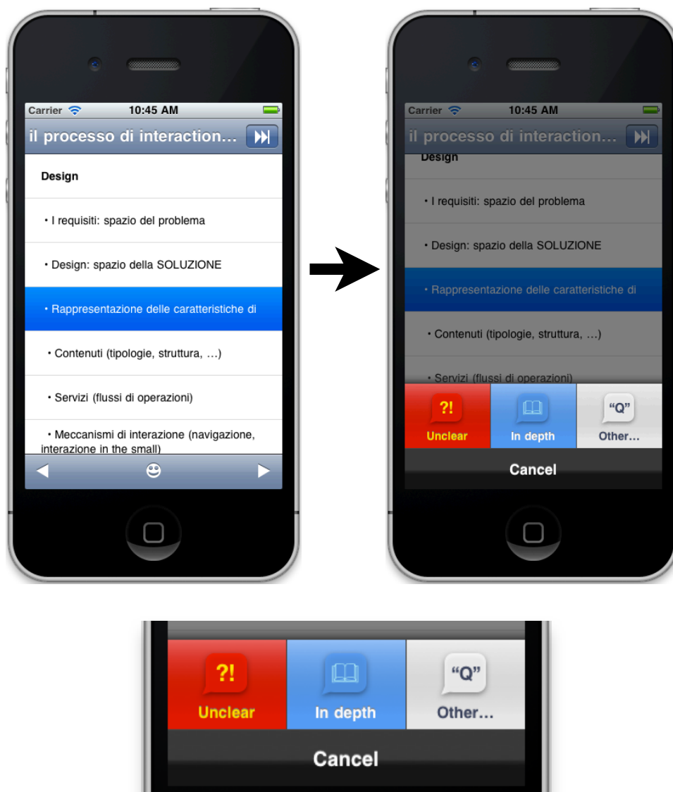
Figure 4.5: Touching a point in the outline view displays the iconographical predefined questions menu.
