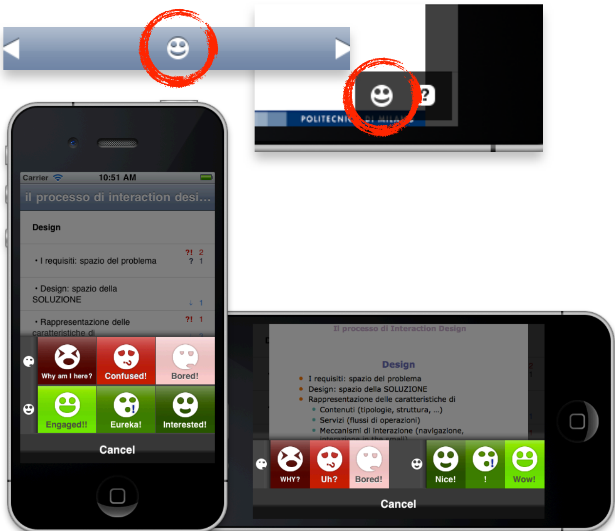
Figure 4.9: The “emoticon” buttons for expressing moods (top left, in the portrait mode toolbar; top right, floating over the slide in landscape mode) open an iconographical menu with several predefined choices.
