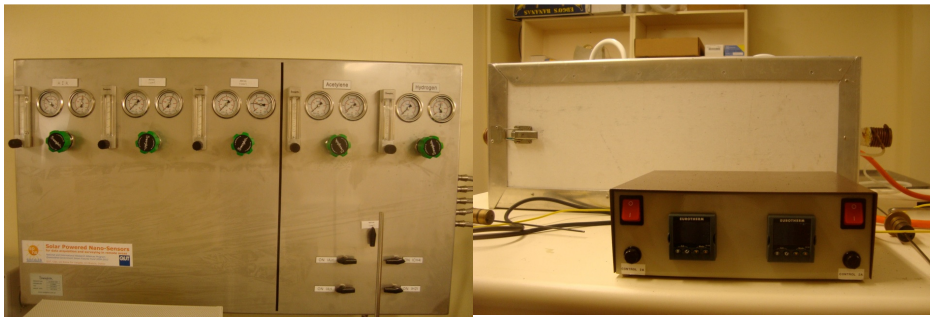
Figure 4.2. Gas flux control (flow measurement sccm ) in the QUT laboratory.
