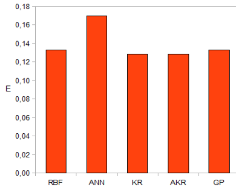
Figure 6.2: Relative test error E_2 on the objective f_2 for different classes of metamodels
