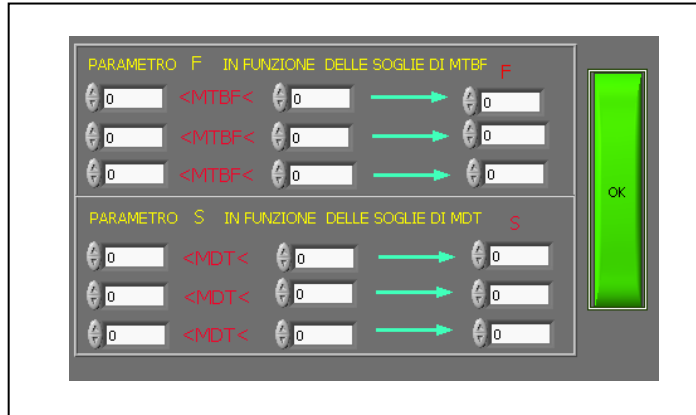
Figure 18. The graphic interface where it is possible to load values about MDT, MTBF and corresponding value of Severity and Frequency
