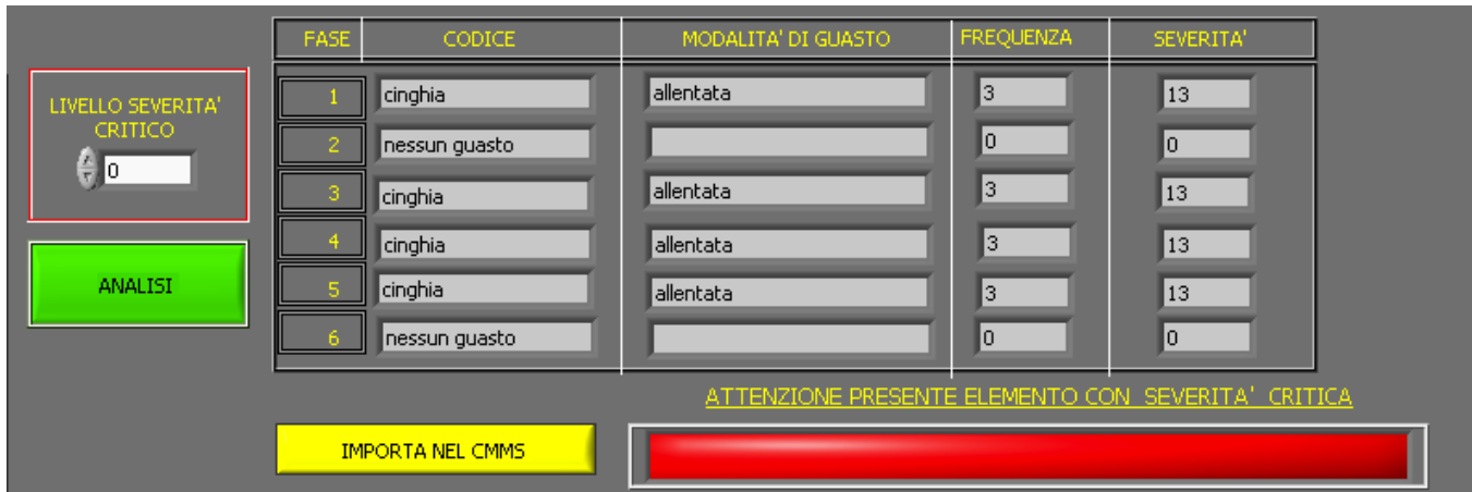
Figure 31: The graphic interface where it is shown the list of faults diagnosed and their associated parameters (failure mode, frequency and severity)
