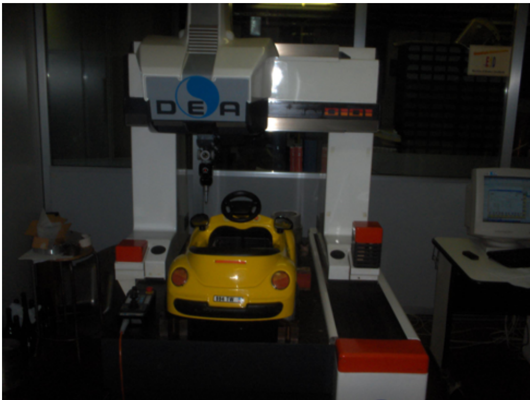
Figure 4.8: Coordinate-Measuring Machine CMM DEA Iota 0101 used at the metrology laboratory of DISPEA, Torino. [Fra+10].
