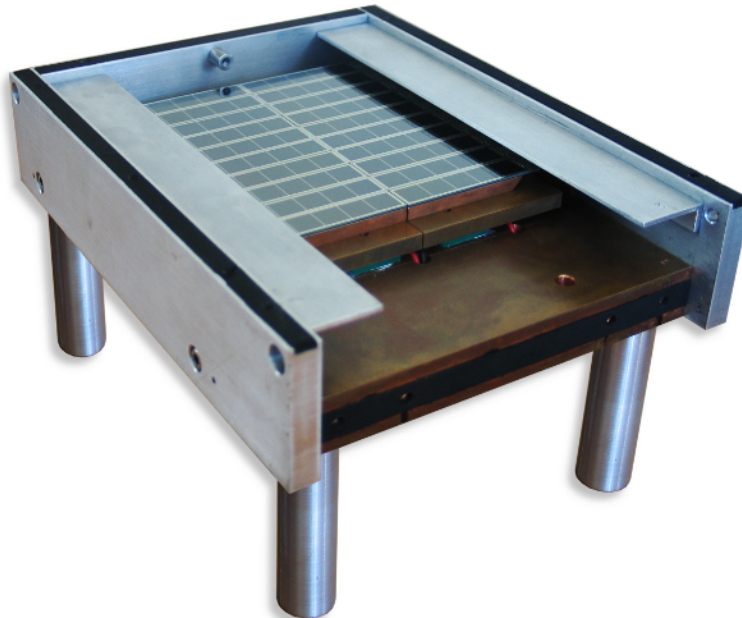
Figure 3.9: Picture of Hicam100 during assembling stages. All the pieces of the case are visible, except for one lateral panel and the cover.
