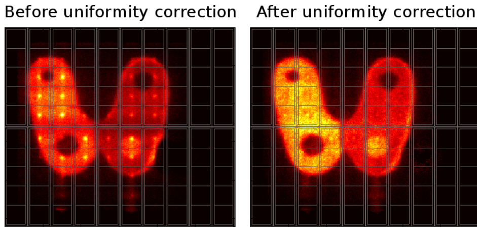
Figure 5.11: Image of a thyroid phantom shown before and after uniformity correction.
